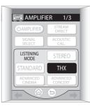
With two channel sources, press **THX** repeatedly to select a matrix-decoding process for the **THX CINEMA** mode (see Listening in surround sound above for an explanation of each process):
